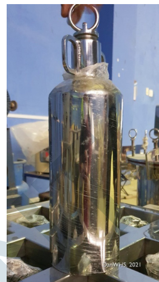
Examples of elemental mercury containers/flask developed by BPPT
