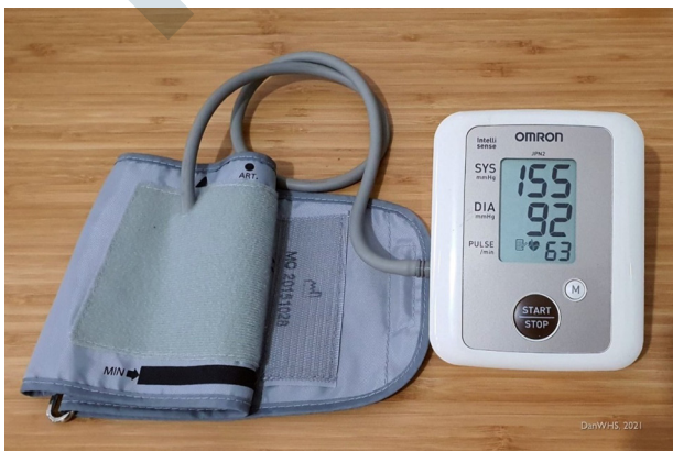
Figure 3.9 Example of A Full-Automatic Blood Pressure Monitor
