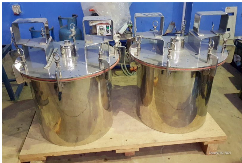
Examples of elemental mercury containers/flask developed by BPPT
